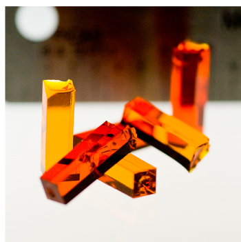
Figure 1. Optically transparent Cr VI /SiO 2 sol–gel monoliths, fabricated by sol–gel chemistry for use in ethylene polymerization experiments.
